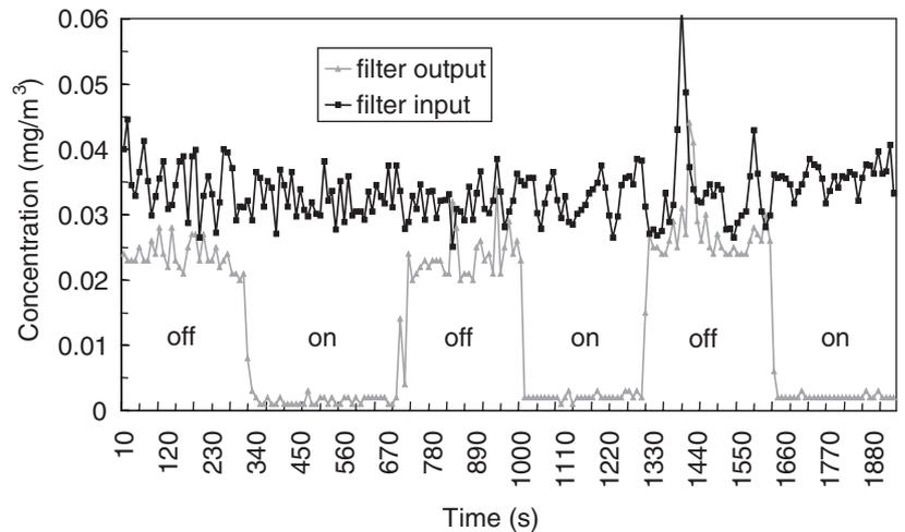
**Fig. 4.** Particles concentrations monitored upstream and downstream of the electrostatic filter (power OFF and ON).
