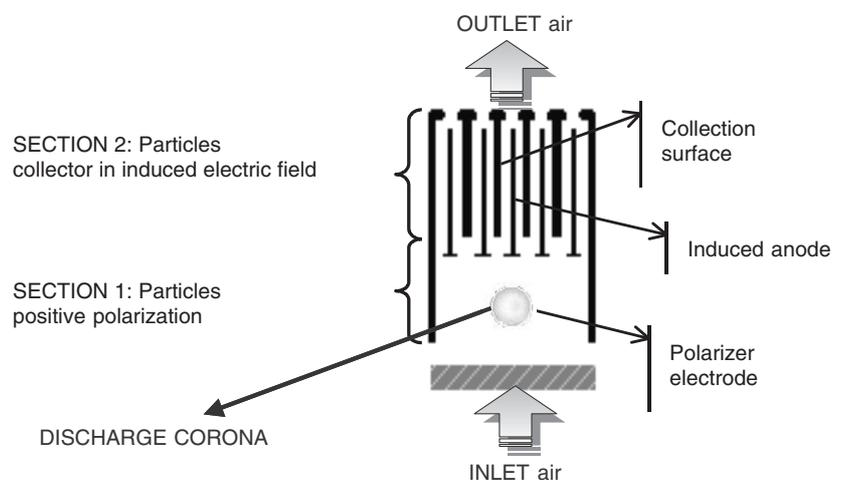
Fig. 1. Electrostatic filter scheme.
