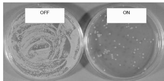
**Fig. 5.** Sampling on the electrostatic filter collection surface. Bacteria showing different growth patterns under conditions of filter OFF and filter ON.
